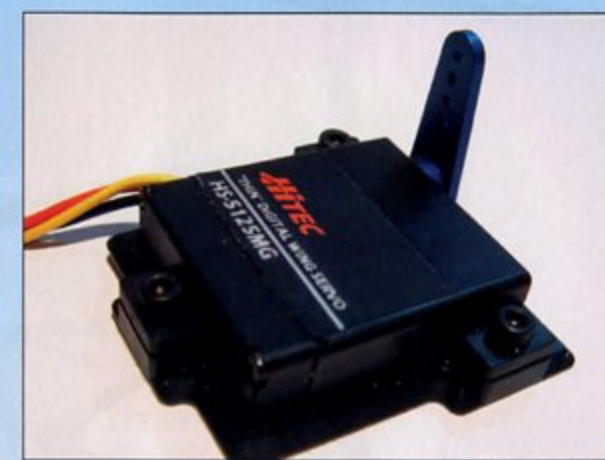
Perhaps the most popular servo for glider wings these days is the HS5125 series. Yep, there's a mount to fit 'em, too.
