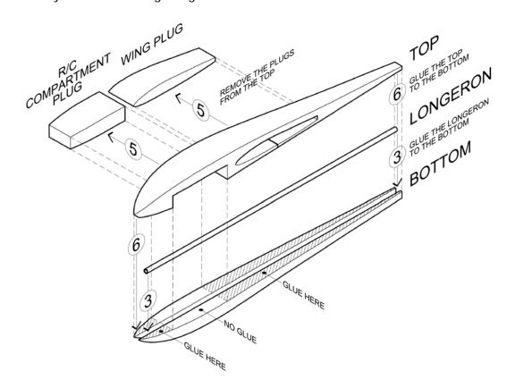
DIAGRAM 4 - FUSELAGE ASSEMBLY
