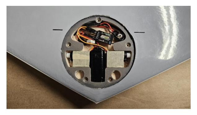
Once you have everything fitted, it's time to close the hatches so you can install the control rods and balance the Wabbit.
